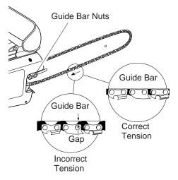
Figure 6 - Saw Chain Adjustment
